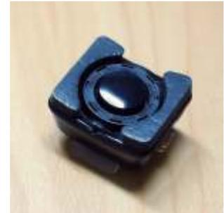
Due to the nature of the device, it provides a high level of ambient noise rejection without the need for electronic noise cancellation. When correctly mounted it provides clear voice communications in ambient noise levels of up to 120dB SPL.
